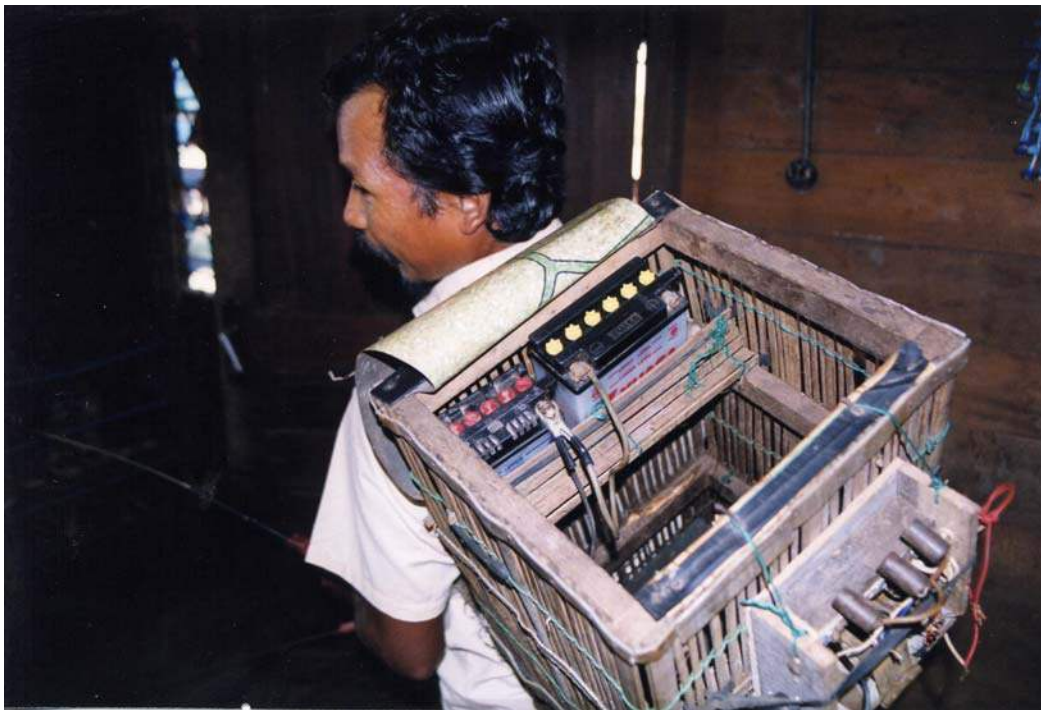
A fisherman wearing the electrical equipment on his back.
